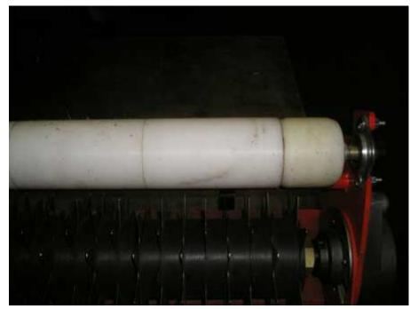
I have taken rolls of hard plastic the same diameter and machined them to fit between the 2 outer rollers of each side. This will keep the units flat and do a much better job when verticutting your fairways.
